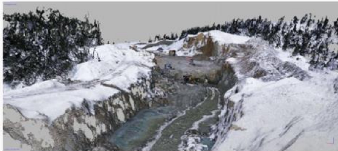
Among other types of outputs, drone data enables detailed point clouds that allow for volume assessment and tracking of road construction.
